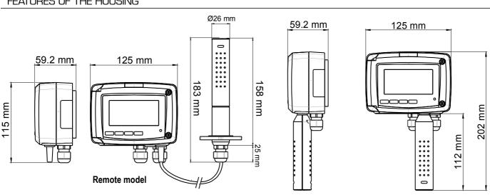
Material: ABS V0 as per UL94 Height of digits: Values: 10 mm; Units: 5 mm
